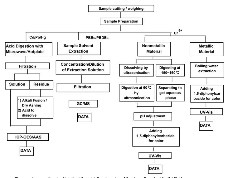
The samples were dissolved totally at the acid digestion step of the above flow chart for Cd,Pb,Hg Section Chief: Gihwan Kim
